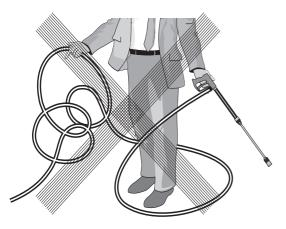
Never pull the high pressure hose if it has formed kinks or "nooses"! Never pull the hose over sharp edges!
