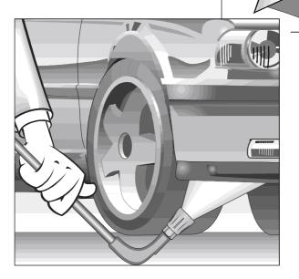
Always aim the underbody lance. Note when using an angled underbody lance, like for example lance no. 41.075 1, that there is a certain amount of torque in the recoil. (Amount of torque 26 Nm)
